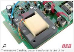
biggest used in a 500-series module. The two inductors are mounted between the transformer and the switches.
