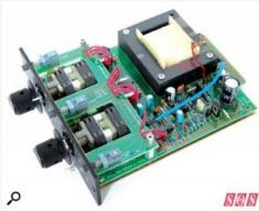
The clean discrete circuitry inside the module creates a very short signal path.
