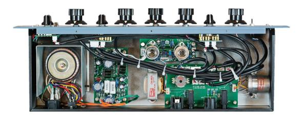
There are three distinct sections of this equalizer comprising low-end shelving Boost and Cut, boost-peaking high-frequencies and high-frequency shelving cut. The Low-Frequency control section offers seven selectable frequency bands at 20, 30, 60, 100, 200, 400 and 800Hz. The old Pultecs, and most other copies feature just four bands from 20 to 100Hz, so this new model has additional control for the lower mid-band.
