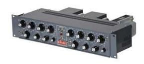
The 2A3 features Pultec-style filters and a switchable highpass filter.
